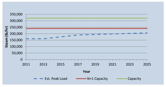
Figure 4-1: Steam Load vs. Capacity
