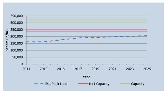
Figure 3-1: Steam Load vs. Capacity
