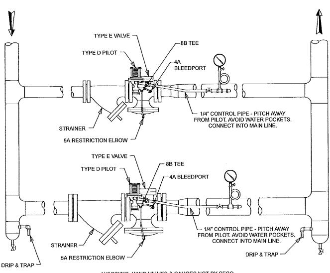
1/4" PIPING, HAND VALVES & GAUGES NOT BY SECO.
